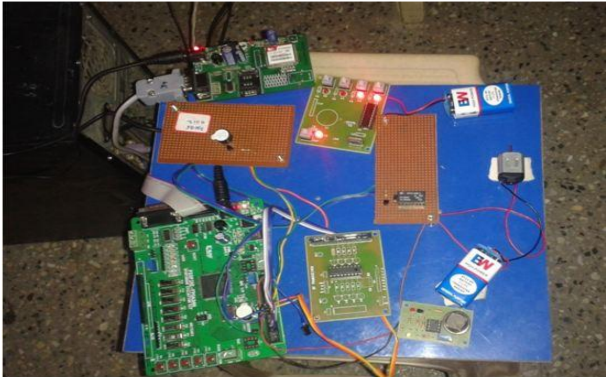
Fig -3: Hardware view of Bus module
