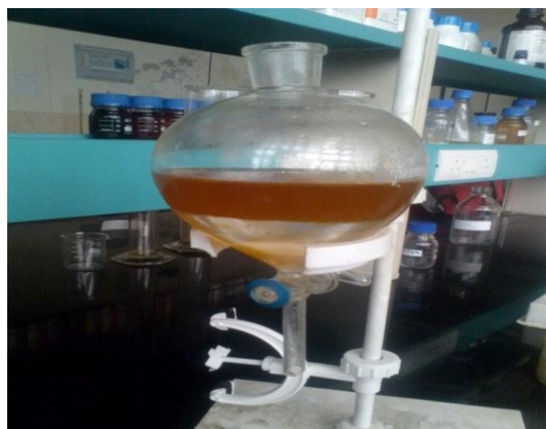
Fig -6: Soap and Glycerol Separation by washing.
