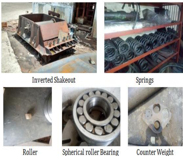
Fig. 5.2: Details of shakeout parts and Bearings
