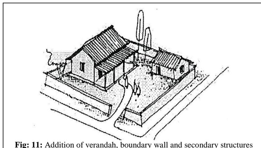
Fig: 11: Addition of verandah, boundary wall and secondary structures
