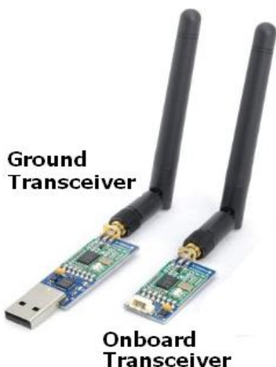
Fig -7: 433MHz lightweight, low power telemetry system is used for ground communication
