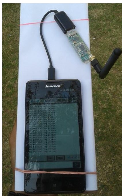
Fig -8: a handheld ground telemetry system is shown with a 433MHz transceiver powered by android phone
