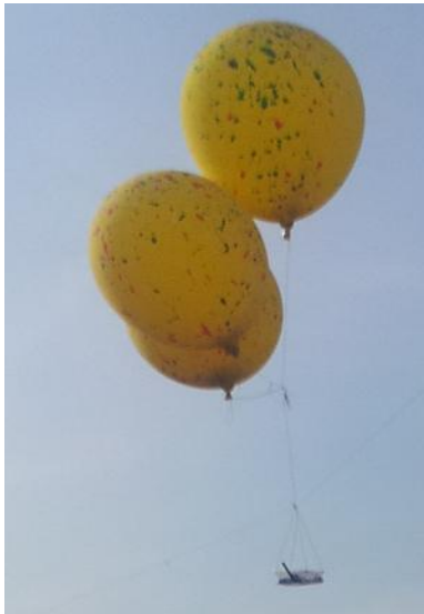
Fig -12: The payload shown in Fig-13 is launched using three hydrogen filled rubber balloons. The ground telemetry system is shown in Fig-8
