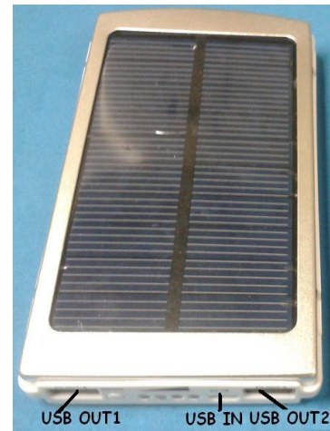
Fig -3: Payload Power Source: a 1.2 ampere-hour solar panel with built-in 10 amp-hour battery having dimensioned same as most Smartphone's
