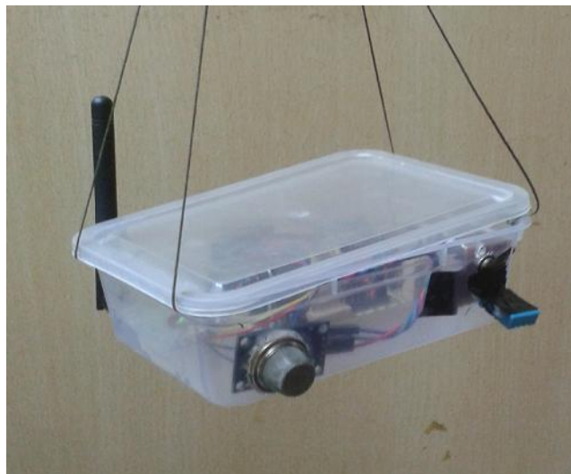
Fig -13: Photograph of integrated balloon payload with sensors, microcontroller, telemetry, 433MHz antenna and power system
