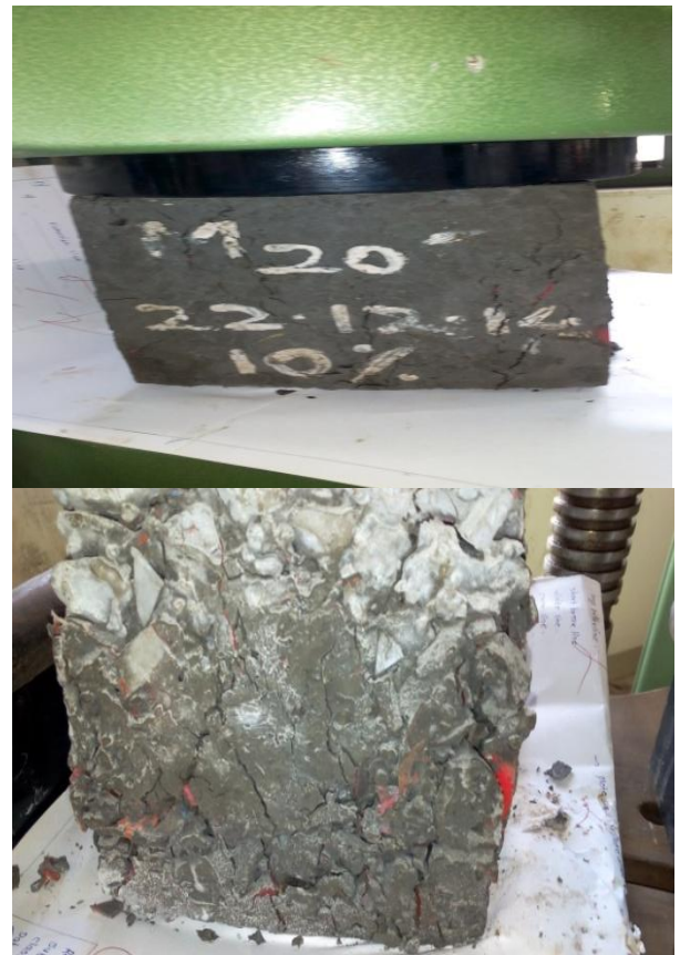
Fig-3: E-Waste block before testing and after testing
