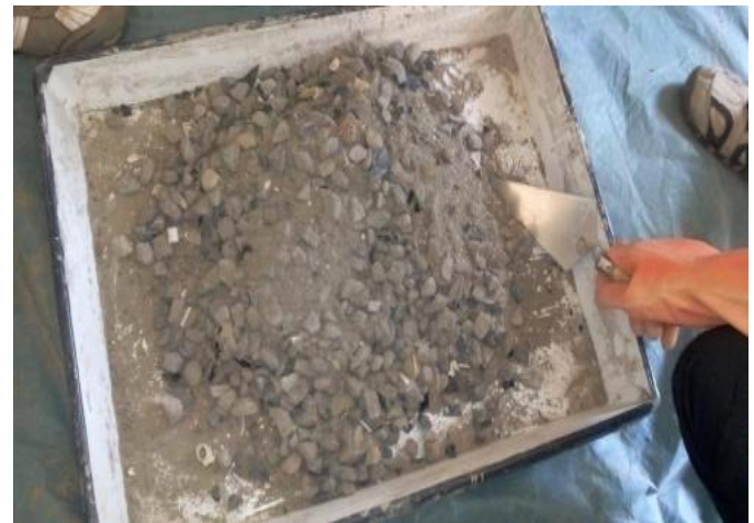
Fig-2: Mixing of e- waste in concrete
