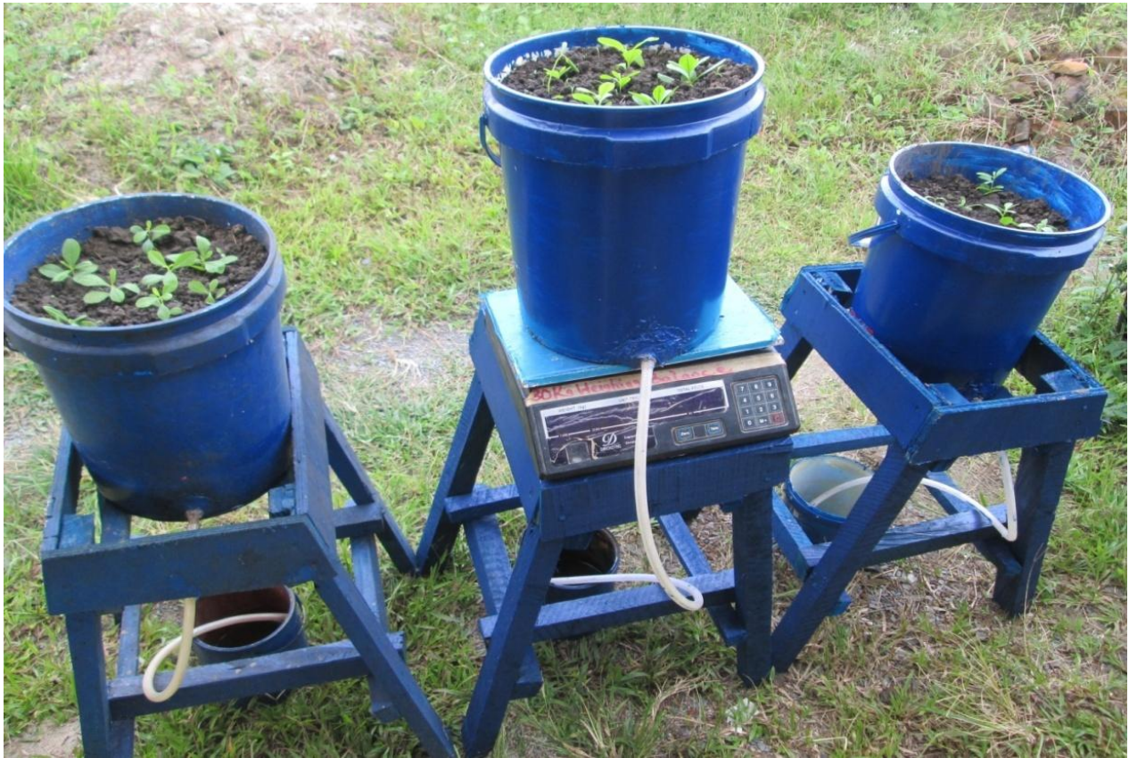
Plate 1: Set-up of the Weighable lysimeter
