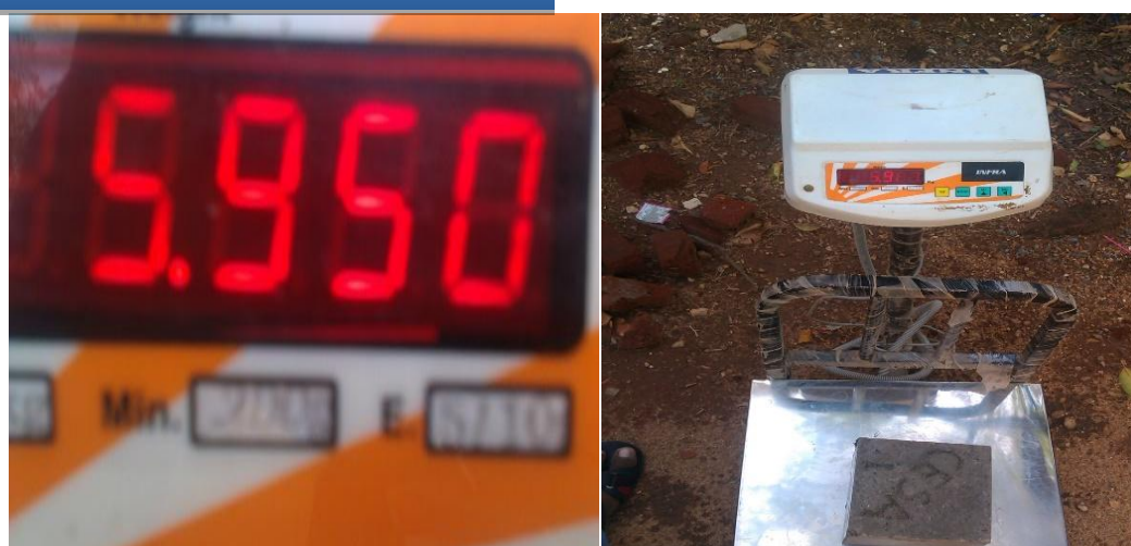
Fig 6: self weight of Vermiculite Concrete cube (light weight For 20% Replacement In Fine Aggregate )
