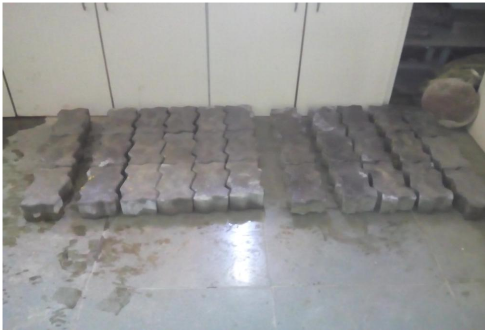
Fig -2: Steel fibers used concrete paving block
