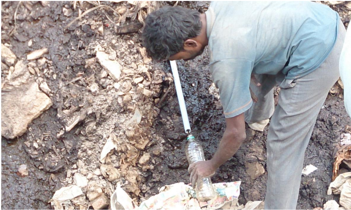
Fig-3 : Process of leachate collection
