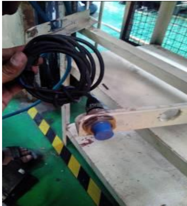
Fig.-5. Fitting of Proximity Sensor according to metal clip Position
