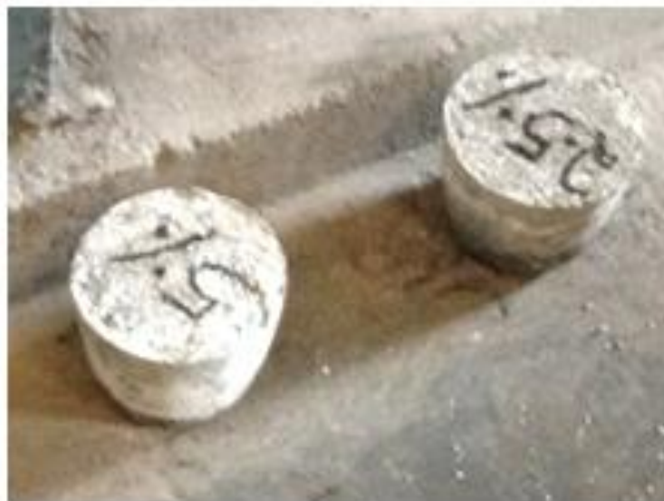
Fig. 2: As cast specimens solidified in the crucible
