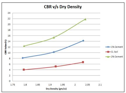
Maximum Dry Density of Soil is 2.052; here consider 97% of Dry Density for determines the CBR value.
