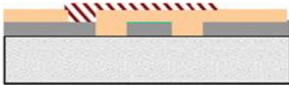
Fig -3.5: Deposition of metal
