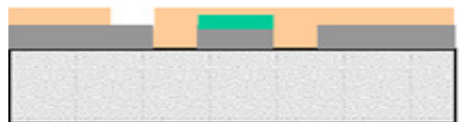
Fig -3.4: Deposition of Sacrificial Layer
