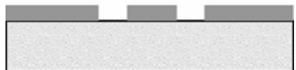
Fig -3.2: Actuated Electrode Formation
