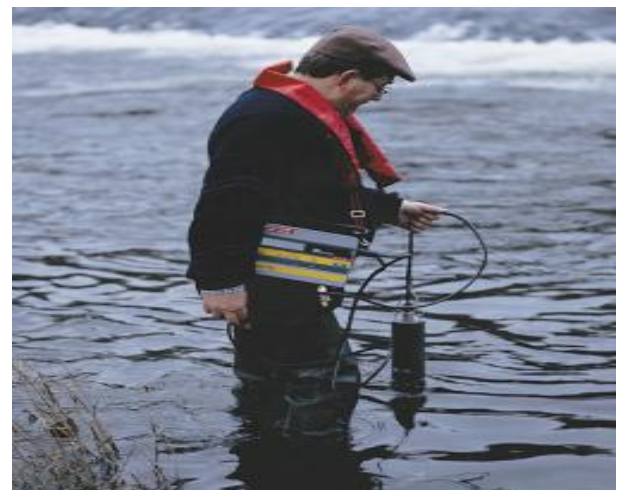
Fig-1: The Previous Methods for measuring Level and Ph balance
