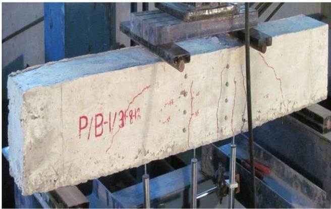
**Fig.-8:** The crack patterns of Reinforced Concrete Beam (i.e. control beams) Specimens
