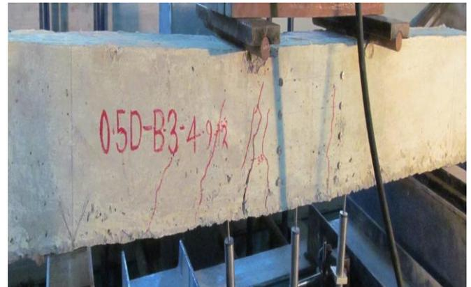
**Fig.-10:** The Crack Patterns of 0.5 Depth Level of Fiber RC beam Specimens
