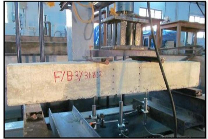
Fig.-7: Beam and LVDT arrangement in 1000 kN Loading Frame
