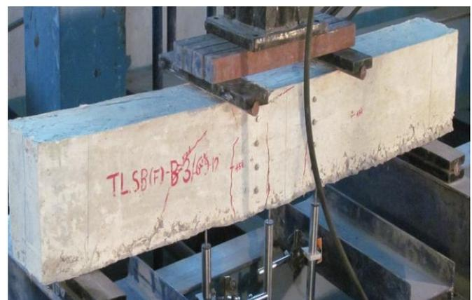
**Fig.-11:** The Crack Patterns of Tensile bar Depth Level of Fiber RC Beam Specimens
