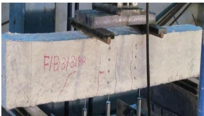
**Fig.-9:** The crack patterns of Fully Fiber RC Beam Specimens
