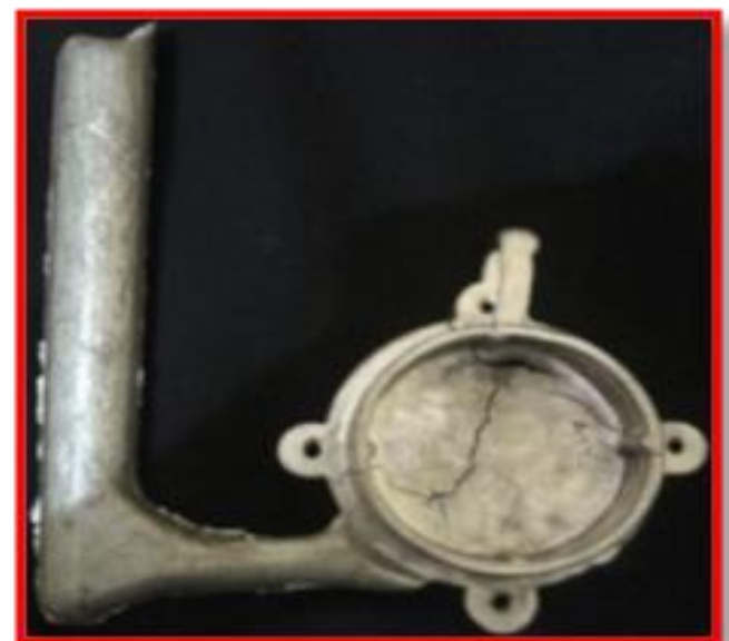
Fig-8a, 8b: Trial-1, Material LM6, Preheat 200°C
