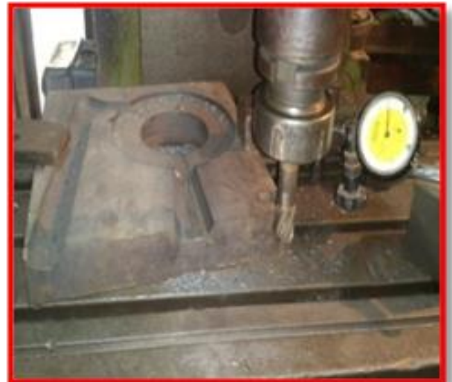
Fig-18: Die during machining
