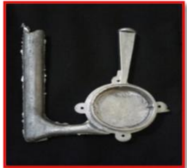
Fig-10a, 10b: Trial-3, Material LM25, Preheat 200°C
