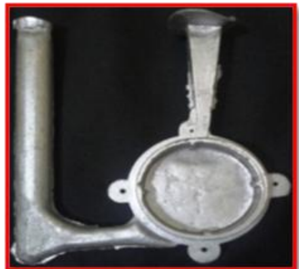
Fig-11a, 11b: Trial-4, Material LM25, Preheat 250°C
