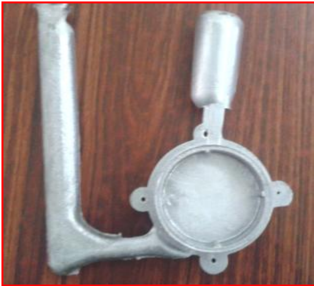
Fig-21: Finally sound casting
