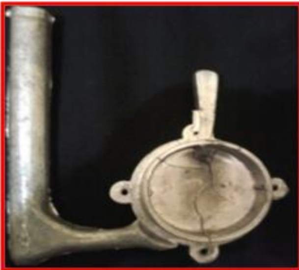
Fig-9a, 9b: Trial-2, Material LM6, Preheat 250°C
