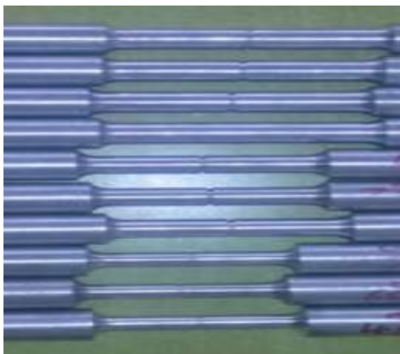
Fig-:2 circumferentially crack round bar testing specimens
