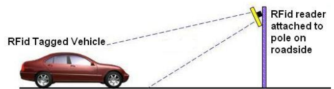
Fig-3: RFID for vehicle detection
