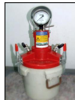
Fig. 5: 8 liters container for the measurement of fresh concrete air content
