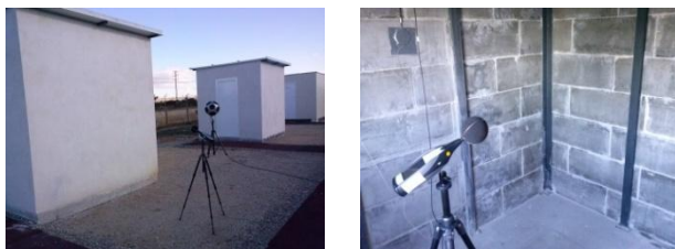
Fig 2 Measurement of airborne sound insulation of façades: sound source (left) and microphone (right).
