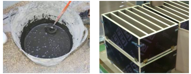
Fig 1 Mixing process (left) and PTFE coated wood molds (right).
