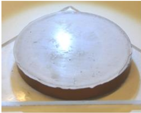
(a) Demolded surface on non-treated grease; shiny reflection
