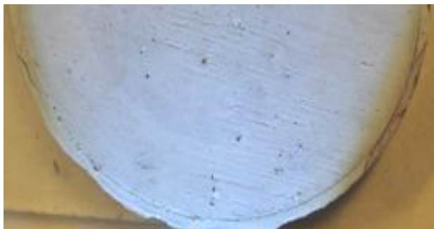
(a) Surface of the hardened cement paste on the non-treated release agent
