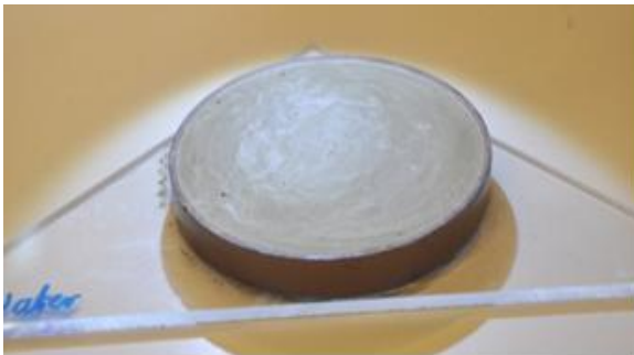
Fig 10: Cylindrical mold on the plastic substrate, filled with cement paste
