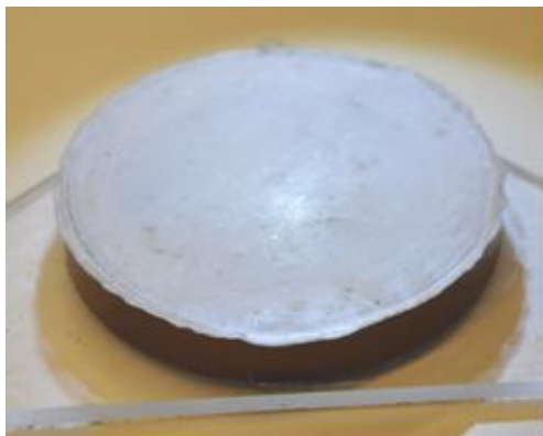
(b) Demolded surface on treated grease; mat reflection
