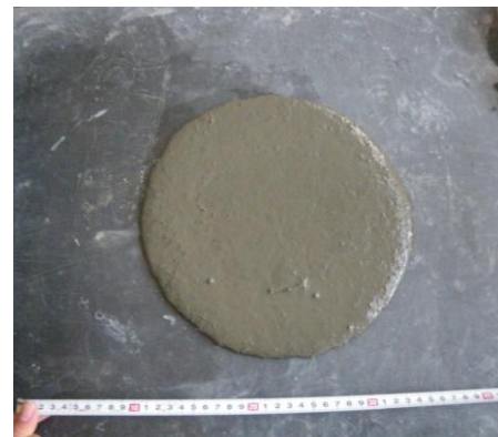
Photo 1: Example of mortar flow (20(5)BS4BS12)
