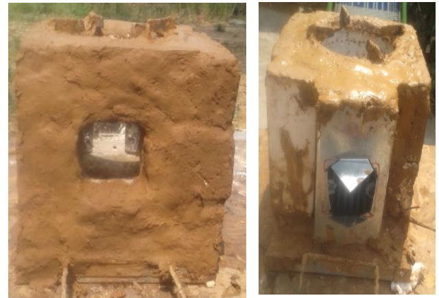
Fig 6: Front and rear view of the TEG integrated improved mud stove.
