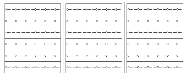
Fig. 3.1 Arrangement of spiked discharge electrode in electrostatic precipitator (Top view)
