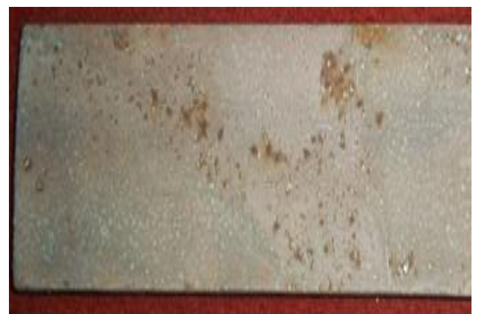
Fig 3.1 Zirconia Ceria Powder (8% \text{Y}_2\text{O}_3 + 67\% \text{ZrO}_2 + 25\% \text{CeO}_2 ) coated samples after salt spray test (358 hours)
