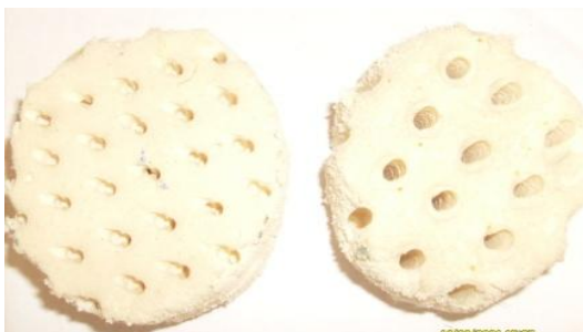
Fig.3. Latex Rubber Foam Sample
