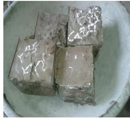
Fig-4: Failure mode of Geopolymer concrete cube
