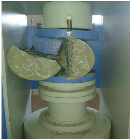
Fig-8: Failure mode of Geopolymer concrete Prism
