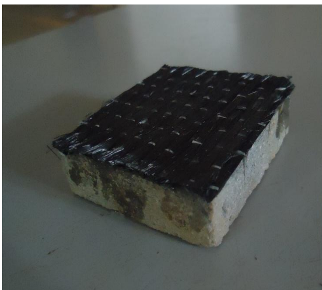
Fig. 1 b 90° CFRP wrapped specimen
