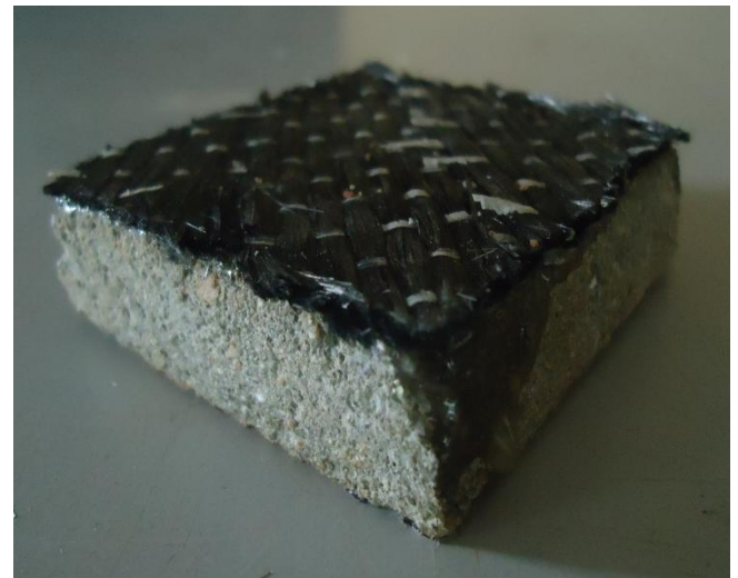
Fig. 1 c 45° CFRP wrapped specimen
