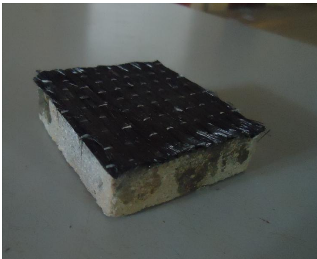
Fig. 1 a 0° CFRP wrapped specimen
