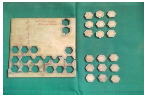
Fig.3.4 Machined specimen of titanium alloy Grade-2 using cryogenic setup
