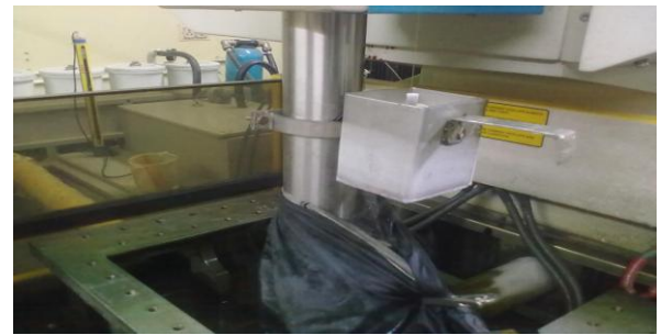
Fig.3.3 Mounting of cryogenic setup on cnc WEDM
