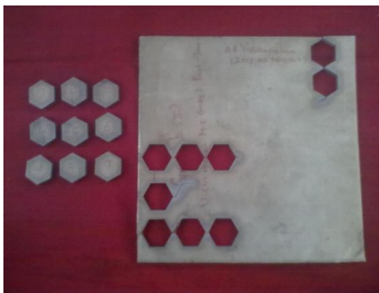
Fig 2.2 machined workpiece on ti alloy (grade2) using normal brass wire
