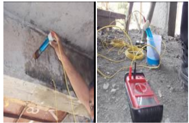
Fig: 1: Set up of half cell potential test
