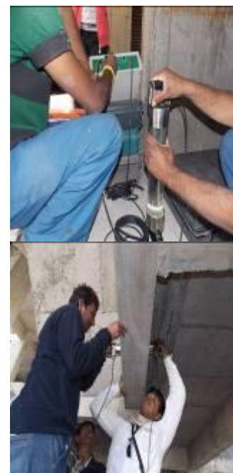
Fig: 2: Calibration and UPV testing of beam
