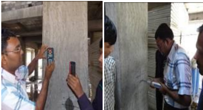
Fig: 3: Rebar locator and rebound hammer
