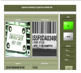
Fig -4: Front Panel for OCR and Barcode Inspection
