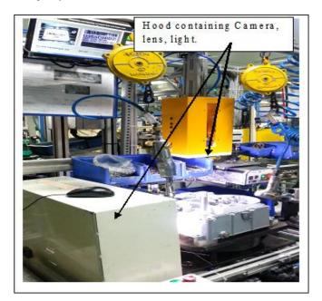
Fig -3: Machine vision setup for Barcode and OCR Reading.
