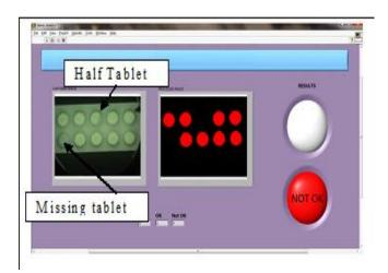
Fig -10: Front Panel for Blister Pack Inspection-showing Missing and half tablets.
