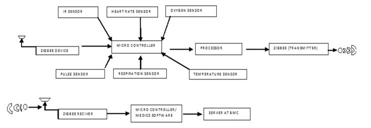
This block diagram gives an rough idea about the working principle of our server. The coordinator node collects the signal altogether and send to the micro controller. The micro controller receive the signals and use the Zig bee module to send all those signals to the Base Monitoring Centre (BMC). Zig bee is the network used here for the transmitting and receiving of signals.
