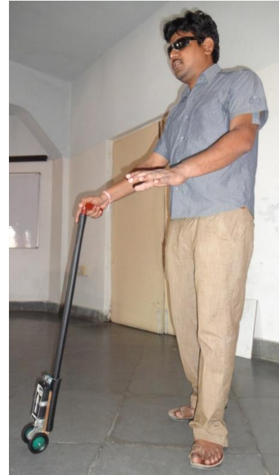
Fig.7 Dual-purpose Blind Navigation Box attached with the motor driving unit and stick is used to hold it.
