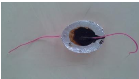
Fig -1: Schottky diode using PANI/Ag nanocomposite
