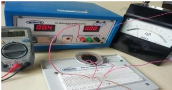
Fig -5: Schottky diode I-V characteristics circuit set-up
