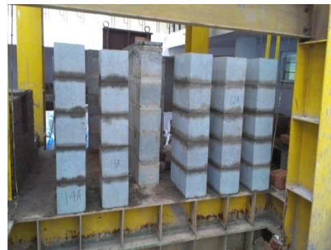
Fig 3(a) Cast prisms on Testing frame
