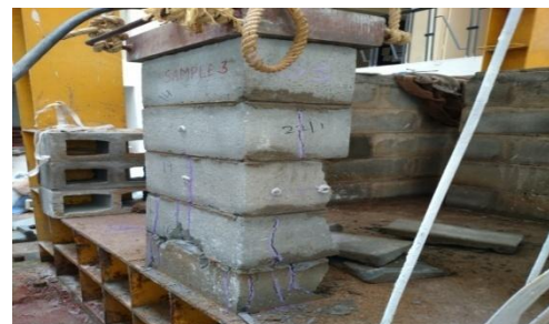
3(c) crack pattern
