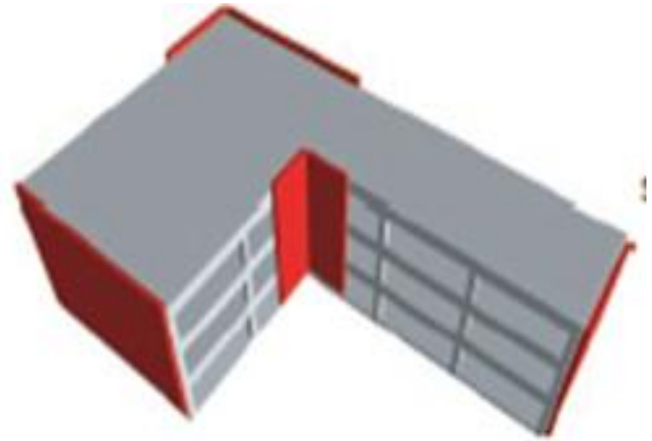
Fig-3: Buildings with Re-entrant Corners Strengthened with Bracings and Shear Walls
