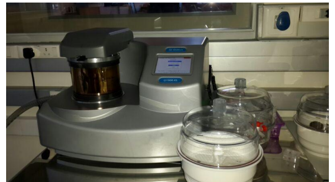
Gold coating after sample preparation before SEM testing[2]
