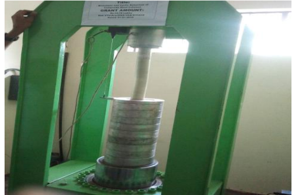
Concrete filled steel tube subjected to monotonic loading [4]
