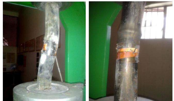
Composite steel tube under testing [4]
