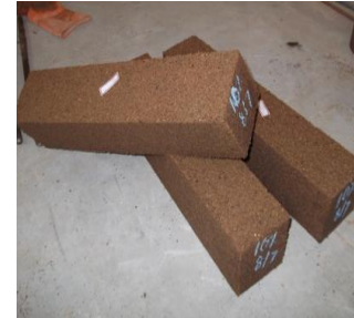
Fig-1: Polymer mortar cubes, cylinders and beam specimens
