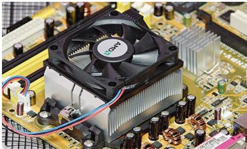
**Fig. 1:** An active (fan cooled) heat sink used for the processor cooling on a PC motherboard
