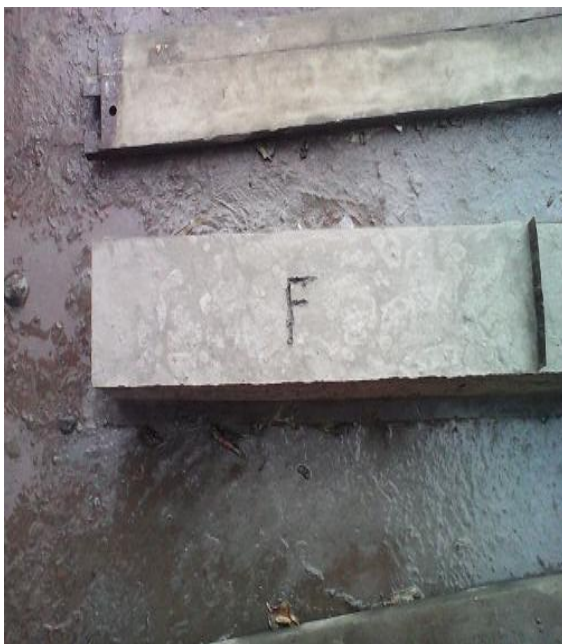
Fig-2: Formwork with beam specimen
