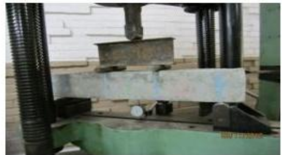
Fig-6: Test Setup to check flexural strength of Beam
