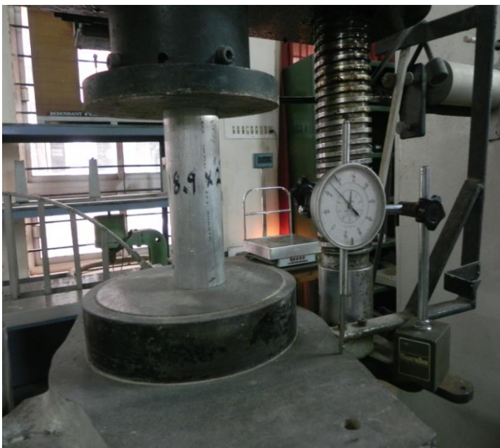
Fig-1: Column axial testing
