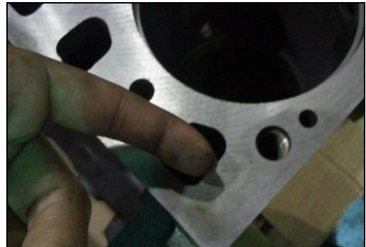
Fig-5: Sand/ metal dust mixture in engine block pockets
