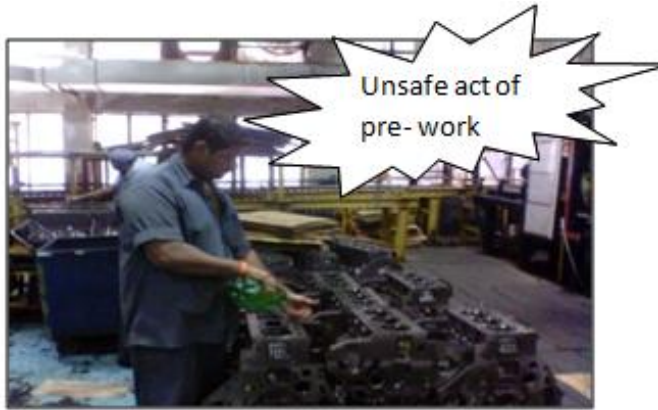
Fig-6: Removal of particulate matter/dust from engine block pockets before final machine block
