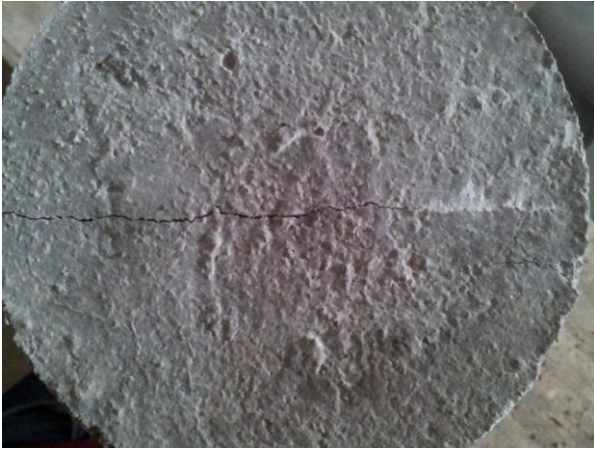
Fig -1: Crack healing in the specimen with bacteria.
