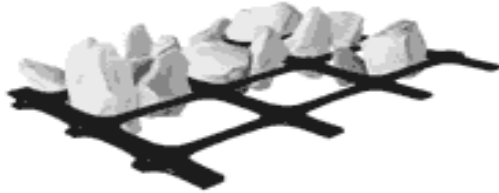
Fig.3 basic mechanism of reinforced earth
