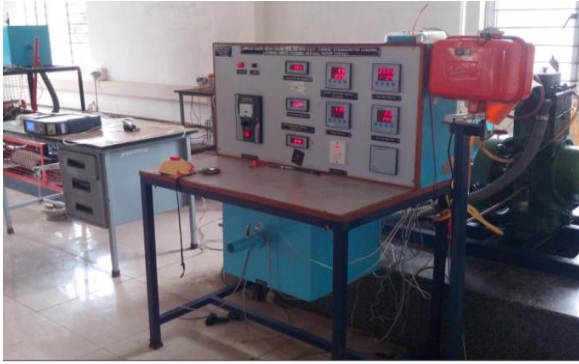
Fig- 2: Diesel Engine Test Rig
