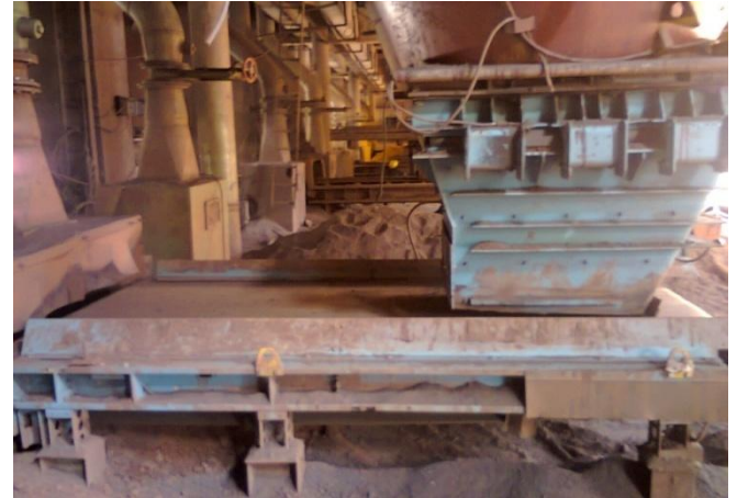
Fig-2: Iron ore weigh feeder
