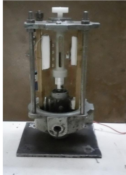
Fig- 1: Centrifuge system used for blood components separation
