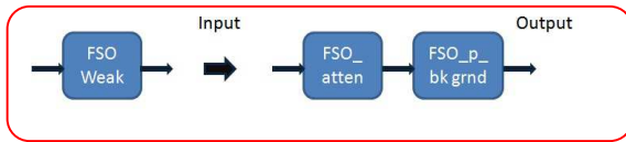
Fig-2: FSO compound component and its internal structure.
