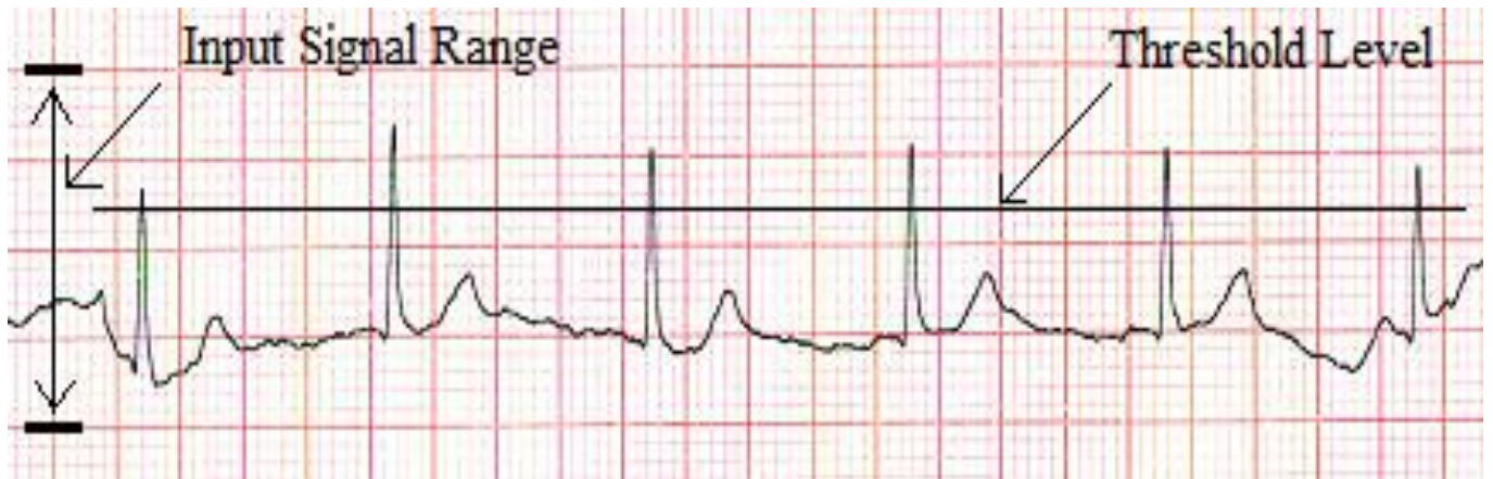
Fig. 3: Input signal range and Threshold level for heart rate calculation
